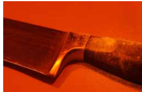
Dusted thumbprint on knife under normal light (top), and under 455nm with orange filter
