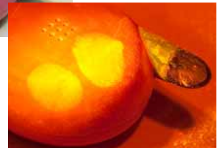
Dusted prints on pink plastic, under normal light (top), and under 455nm with orange filter (bottom).
